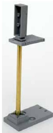
Apply some EPOXY to the post and slide Platform up to meet underside of Back Box and ensure they are in direct contact. **If they are not in direct contact, the support bracket for the route indicator will not fit.** Again, Superglue sets a bit too fast for this operation.
