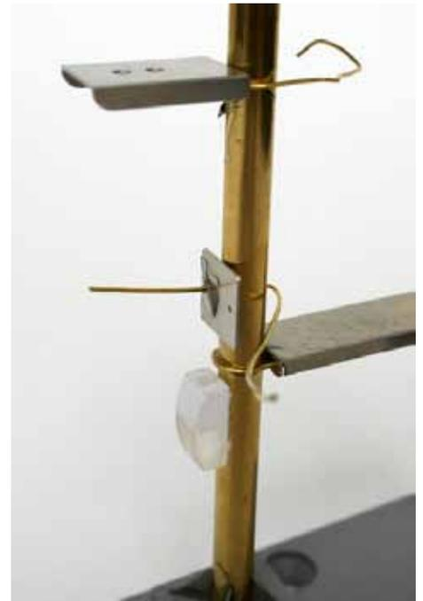
Fit the Route Indicator Support Bracket to the slots in the platform and ensure it is square before glueing – ENSURE the protruding top plate is at the rear and that the centre hole in the plate aligns with the hole in the back box
