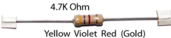
Solder the resistor to the white wire(Positive) and connect to a 12V DC supply and switch
