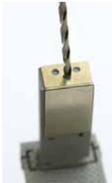
Fitted to an existing signal using the jig to mark the wire hole.
