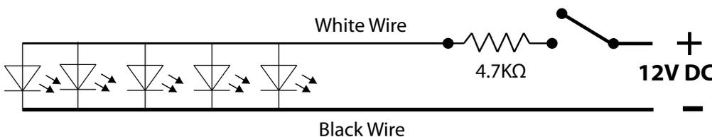
This signal can be used with digital control devices but use the supplied resistor as well even if the instructions say that resistors are built-in.
